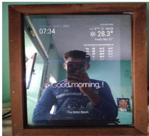
Fig. 2. Intelligent mirror shows date, time, and weather.
